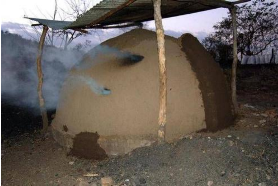
Figure 27: Test of high efficiency kiln for charcoal production in the ECO CARBON FRA facility in Nagarote Municipality, provided by MEM with support from ESMAP.
